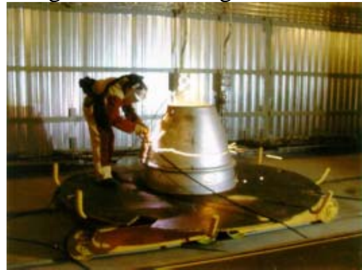
Cutting up an SS-18 nozzle
