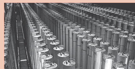
IR-1 centrifuges; about 1,000 of such centrifuges at the Natanz enrichment facility were disabled by the Stuxnet virus. Photo: Russian Atomic Community
