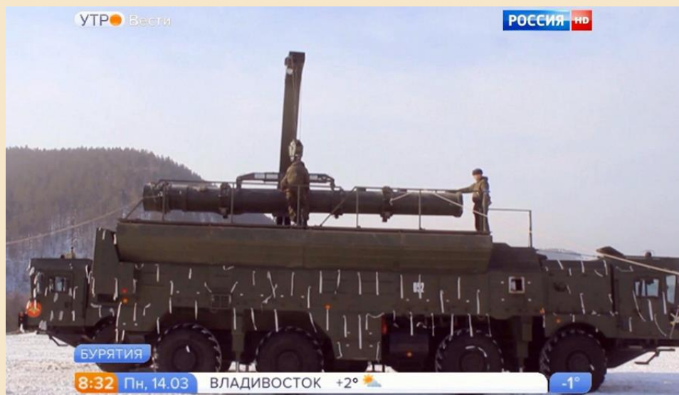
Image 1. Loading a launch tube into the Iskander-M TEL. Source: Youtube
